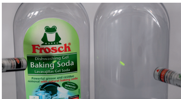
A specific IR laser pointer makes the fluorescence visible. The marker can be inserted in the label (left) or in the plastic itself (right).
