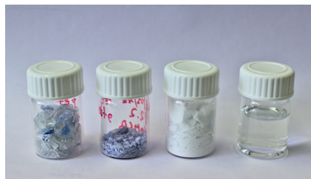
From PET to its basic components terephthalic acid (TPA) and monoethylene glycol (MEG)
